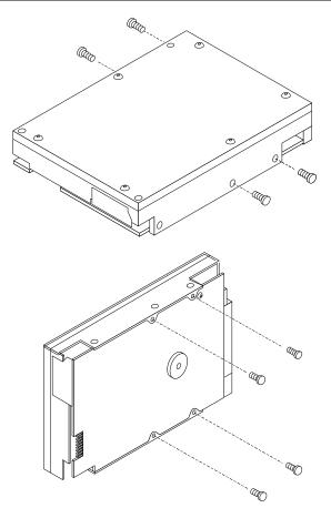
Figure 2. Mounting holes
