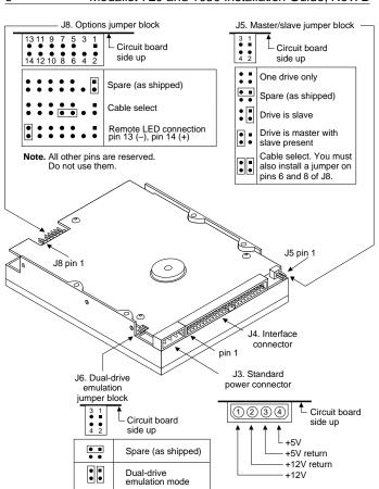
Figure 1. Jumpers and connectors
